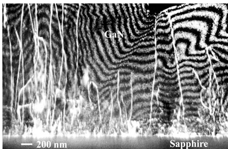
Figure 5. Weak beam image ( g = 0002 ) of WB 42 showing the distribution of threading dislocations.
